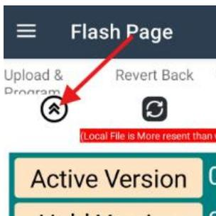
4. Select “**Yes**” to flash device. A progress bar will indicate the download and flashing process
